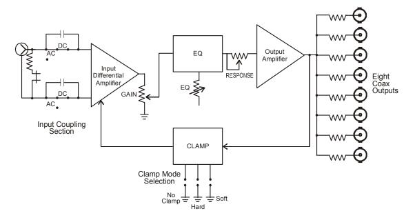
Figure 7-1. VEA-6840 Functional Block Diagram
